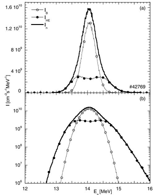
**Fig. 4.** The neutron spectrum and its B and HE components giving the best fit to measured spectrum of the neutron emission from the RF heated discharge JET #42769 in linear (a) and (b) log scale plots.
