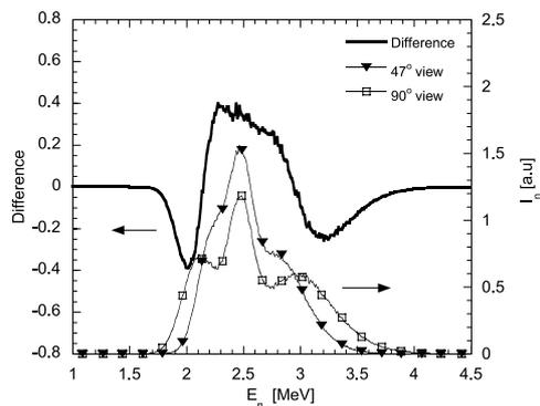
**Fig. 10.** Calculated difference spectrum for the 2.5-MeV neutron emission from D plasma subjected to ICRH derived from the results in Figures 6 and 8 representing observations at  $\theta_{view} = 47^\circ$  and  $\theta_{view} = 90^\circ$ .
