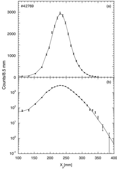
**Fig. 2.** Measured proton recoil histogram reflecting the spectrum of the neutron emission from the RF heated discharge JET #42769 plotted on (a) linear and (b) log scale;  $X_p$  is the position on the MPR focal plane detector having an energy dispersion of about 10 keV/mm. The full line is a fit to the data points using the model described in the text.
