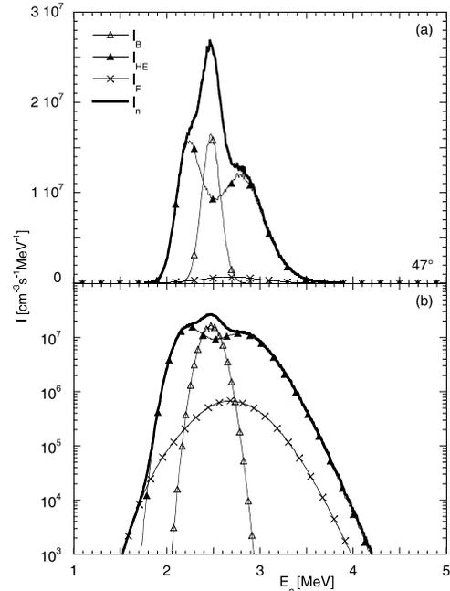
**Fig. 6.** The projected neutron spectrum for neutron emission from  $dd$  reactions in RF heated discharge of plasma conditions equivalent to those derived from neutron data for the DT discharge JET #42769 in (a) linear and (b) log scale plots; the bulk ( $I_B$ ), high energy ( $I_{HE}$ ) and fast ( $I_F$ ) components are shown as well as the sum ( $I_n$ ).
